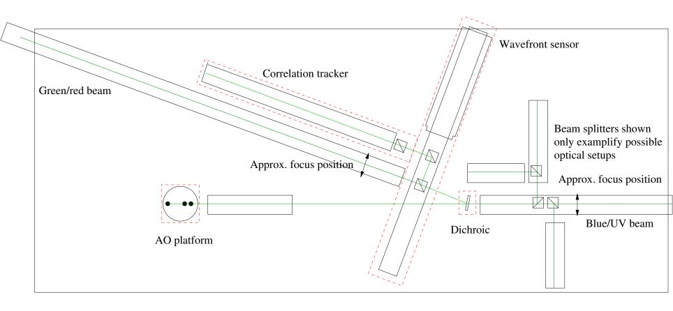
Optics and opto-mechanics within dashed lines must not be moved or adjusted
